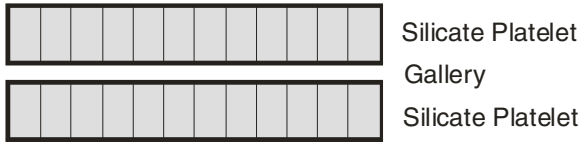
Fig. 1 Idealized layered silicate structure
