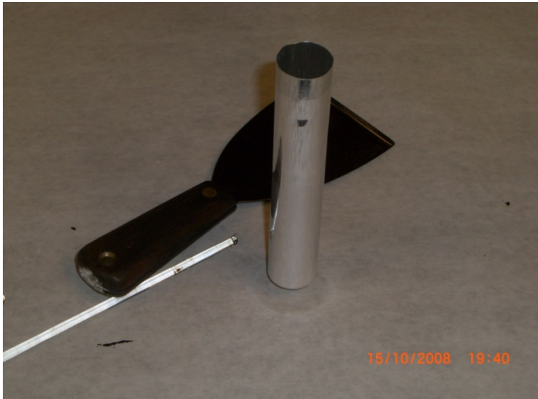
Fig. 1 The separation tube used in the dispersion analysis
